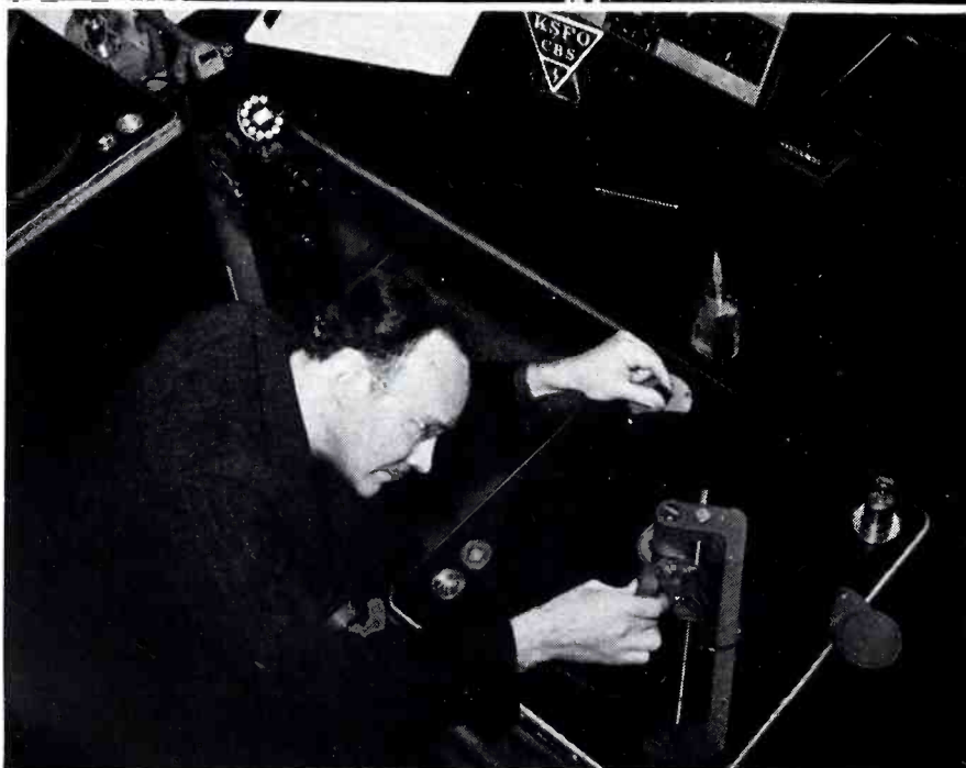
LEFT: Merrill DeWitt, KSFO Engineer in Charge of Recording, using the 72-A recorder attached to the 70-A turntable.
