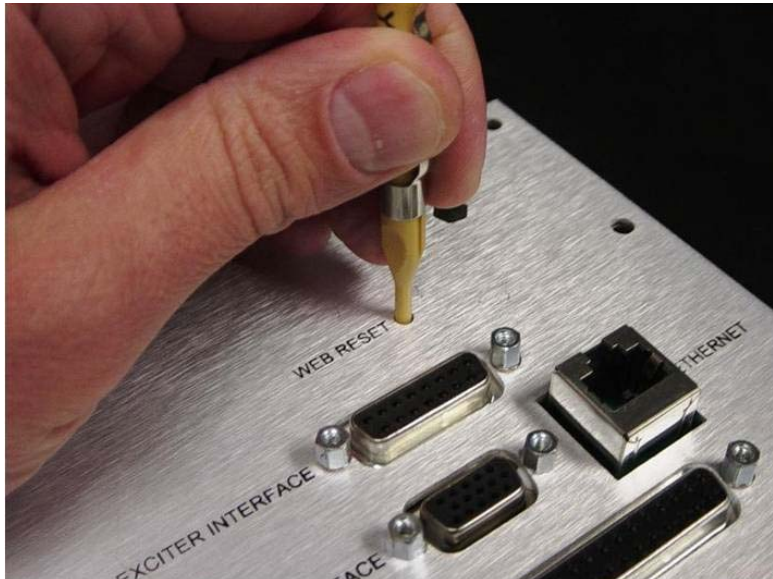
Figure A-6 Reset of web remote via WEB RESET hole on I/O panel.
