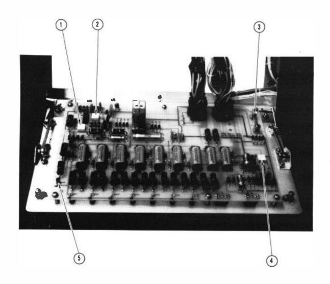
Figure 3-3. Cabinet 1 Fault and Overload Assembly Printed-Circuit Board Controls and Indicators
