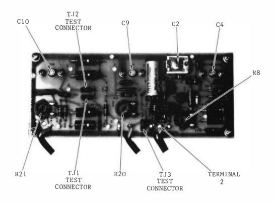
Figure 5-4. Directional Coupler 2Al Adjustment Locations
