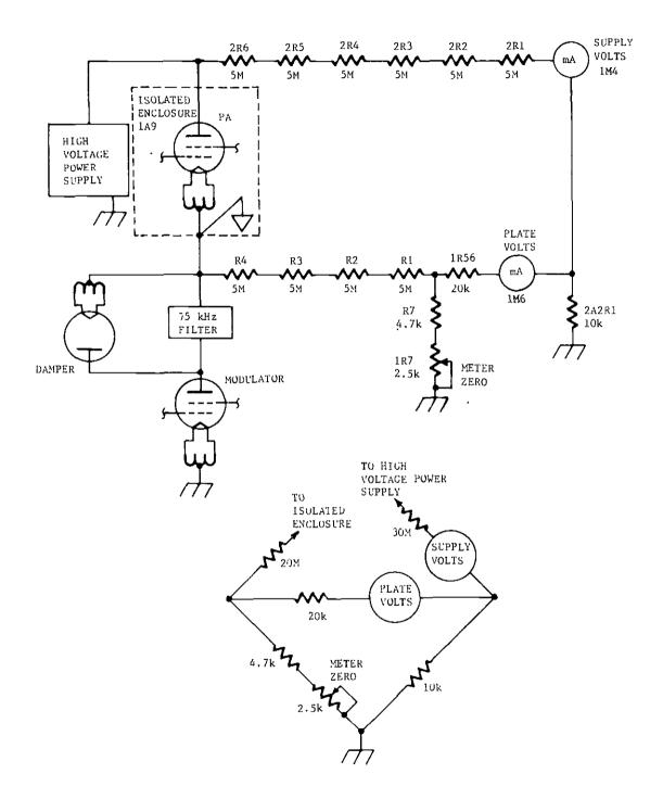
Figure 4-11. High Voltage Metering
