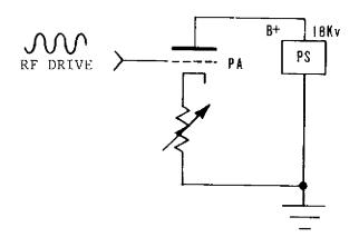
Figure 4-2. PDM Equivalent Circuit
