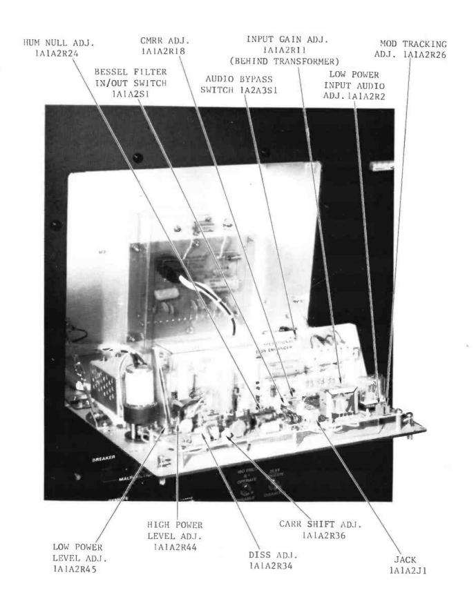
Figure 2-24. PDM Controls
