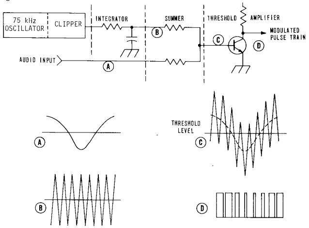
Figure 4-4. MW-50C3 Transmitter PDM
