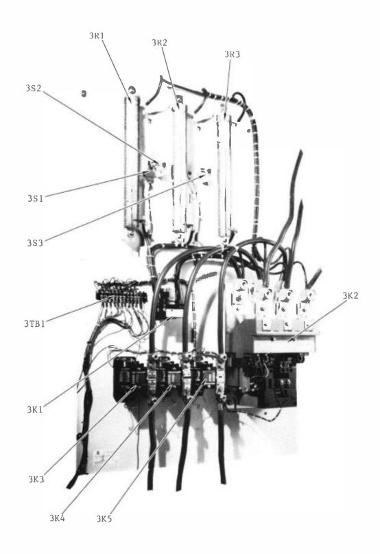
Figure 2-16. High-Voltage Step-Start Assembly
