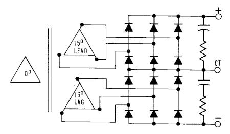
Figure 4-5. 12-Phase Circuit
