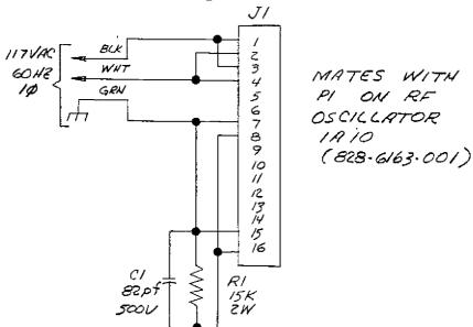
Figure 5-1. Oscillator Unit Bench Test Cable
