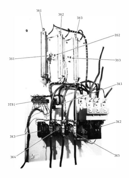
Figure 1-2. High-Voltage Step/Start Assembly
