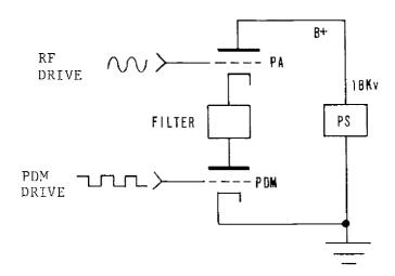
Figure 4-3. PDM Simplified Circuit
