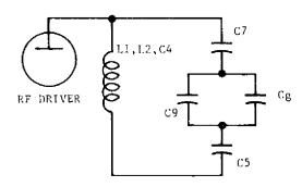
Figure 4-7. RF Driver Plate Circuit
