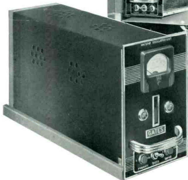
On the left is shown one of the frequency control units removed from the transmitter. Each one contains a complete oscillator and first buffer with crystal and oven. The thermometer on the crystal oven can be viewed thru the vertical slot on the front. Tuning controls and switch for changing the meter from the plate circuit of the oscillator to that of the buffer are located at the bottom of the panel.
