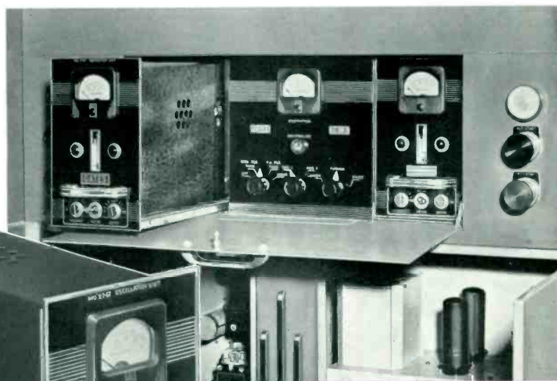
Above is the "Customaire" showing front doors open and wide accessibility to tubes and relays. At the right is a close-up of the frequency control unit section. One control unit is shown partially removed. On the center panel are the tuning controls for the entire transmitter. The center switch selects either control unit, the left switch designates which circuit is being tuned and the right switch shows direction of the adjustment being made. The meter indicates grid current to the 813 exciter stage.
