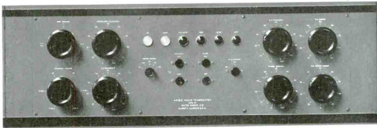
All functions are clearly indicated on the control panel section of the HF-8 transmitter.
