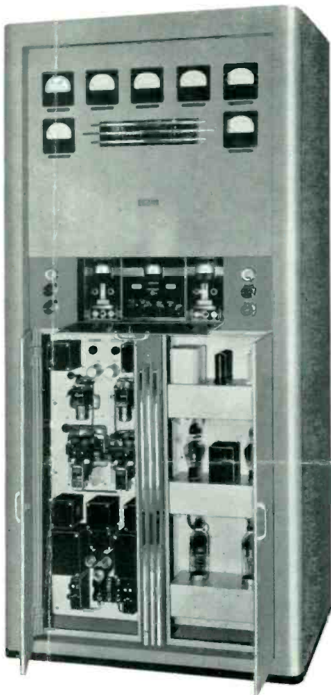
Above is the "Customaire" showing front doors open and wide accessibility to tubes and relays. At the right is a close-up of the frequency control unit section. One control unit is shown partially removed. On the center panel are the tuning controls for the entire transmitter. The center switch selects either control unit, the left switch designates which circuit is being tuned and the right switch shows direction of the adjustment being made. The meter indicates grid current to the 813 exciter stage.
