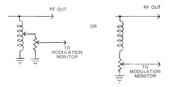
CONNECTIONS FOR AN ADJUSTMENT PICKUP COIL
